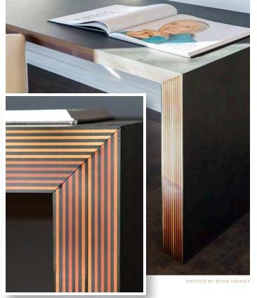
Two 1<sup>1</sup>/<sub>4</sub>-inch panels were fastened together to create the 2<sup>1</sup>/<sub>2</sub>-inchthick desk, with the black paper as the top and the edge revealing the alternate layers of black and bleached. That reveal follows a theme seen in several other places in the house, including the fireplace.
