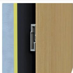
Concealed Fastener Installation
